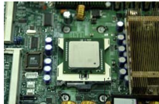
Socket lever in the locking Position
